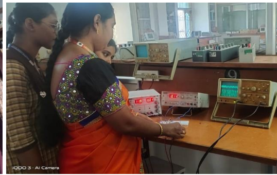
Figure 2: Practical Realization of CE Amplifier Using Breadboard Trainer
